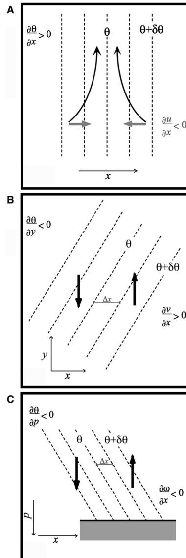
**Fig. 7** (A) Confluent horizontal flow acting on meridionally oriented isentropes. The gray arrows represent the  $x$ -direction wind. (B) Effect of horizontal shear on  $\frac{\partial \theta}{\partial x}$ . The black arrows represent the  $y$ -direction wind. (C) Effect of tilting on  $\frac{\partial \theta}{\partial x}$ . The black arrows represent upward and downward vertical motions.
