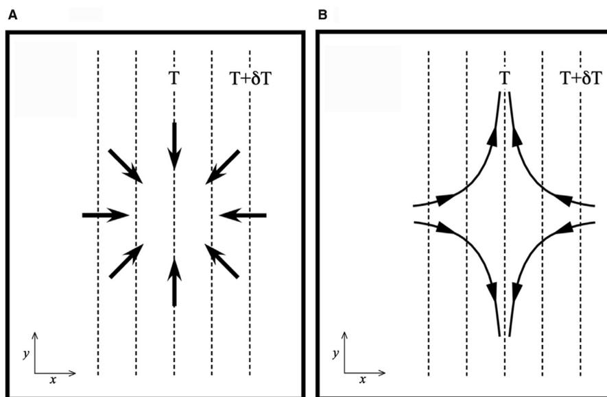
**Fig. 5** (A) Pure convergence superimposed upon a field of isotherms. (B) Horizontal deformation superimposed upon a field of isotherms. In both cases the horizontal wind will tend to intensify  $|\nabla T|$ . Adapted from [Martin \(2006\)](#).
