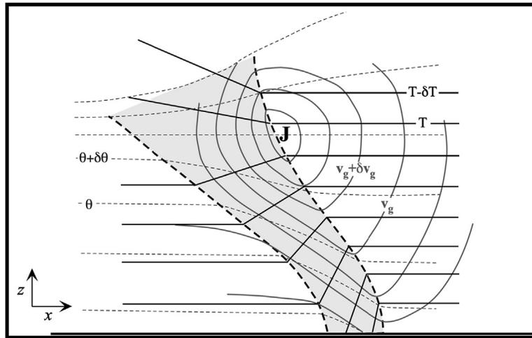
**Fig. 4** Idealized vertical cross-section through a frontal zone. Gray solid lines are isotachs of the geostrophic wind into the page with “J” indicating the position of the wind maxima. Black solid lines are isotherms and thin dashed lines are isen-tropes. Gray shaded region with thick dashed border represents the idealized frontal zone. Adapted from [Martin \(2006\)](#).
