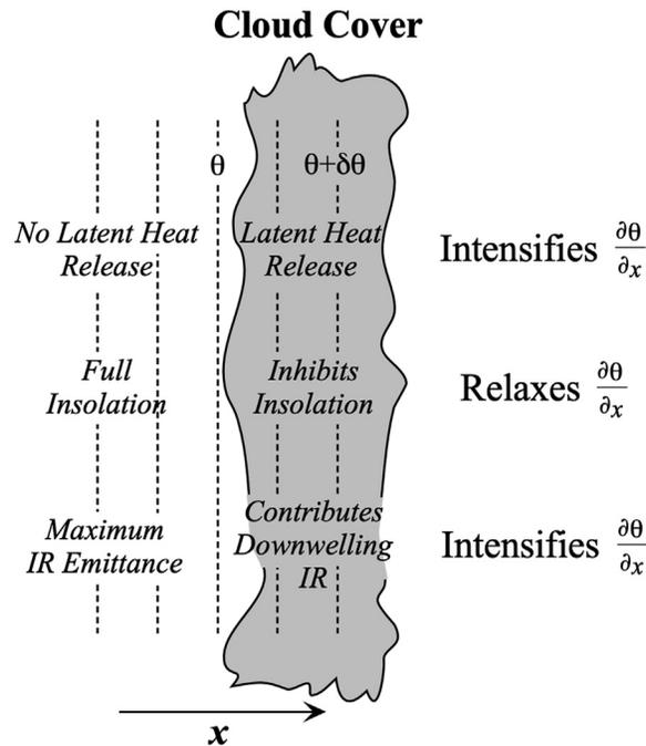
**Fig. 6** The diabatic effects of cloud cover on  $\frac{\partial\theta}{\partial x}$ . The effect of differential latent heat release can occur at any time of day. Differential insolation and IR emittance are specific to day and night, respectively. Adapted from Martin (2006).
